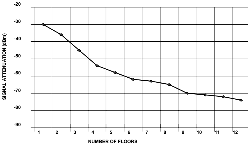
FIGURE 6.16 Path loss between building floors.
