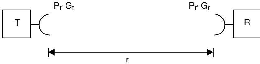
FIGURE 20.4 Transmitting and receiving antennas in free space.
