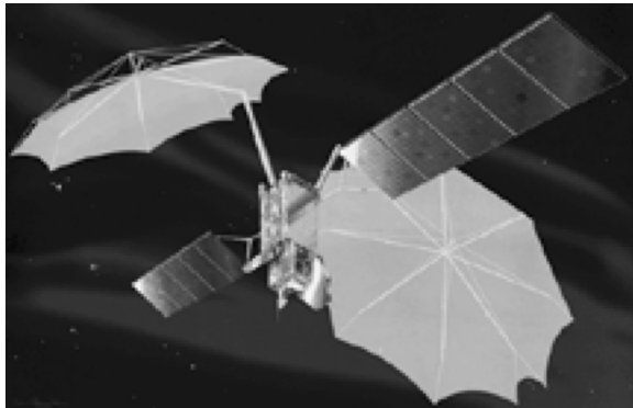
FIGURE 9.13 ACeS spacecraft: deployed.
